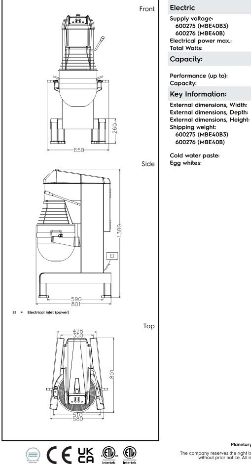
655 mm 850 mm 1370 mm 204 kg 203 kg ISO 9001; ISO 14001 kg with Spiral hook
